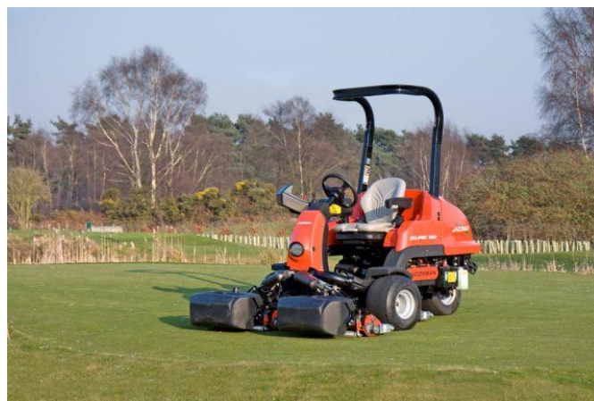
The Jacobsen Eclipse 322, a diesel-electric hybrid riding greens mower
